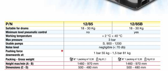
\* theoretical valves, friction coefficient has not been considered. Furthermore depression's force created by the pump during suction (+2100 Kg) must be added to the listed figures.
