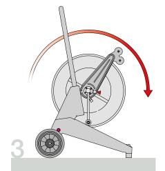
Slowly release the handle until the trolley is resting completely on the ground: the super block system is activated automatically.
