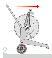
Tilt the handle further back and move the trolley in the desired direction.
