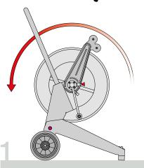
Tilt the handle downward: the super block system is automatically deactivated, but the trolley is still touching the ground.
